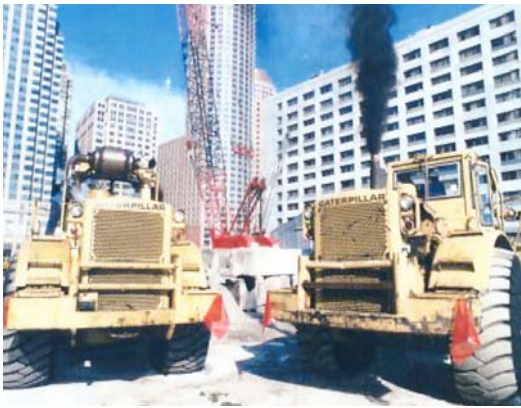
After and before retrofit, at Boston's Big Dig.
